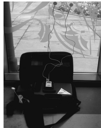
Fig. 1 Contact microphone attached to window
