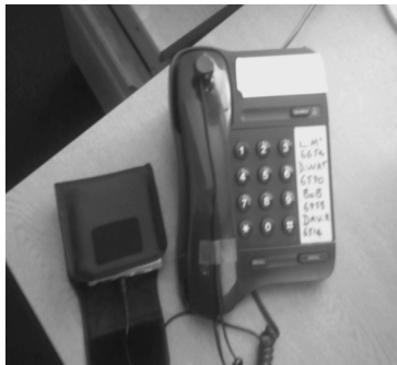
Fig. 2 Electromagnetic Coil attached to office telephone
