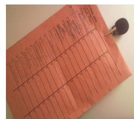
Fig. 3 internal mail envelope with attached microphone.
